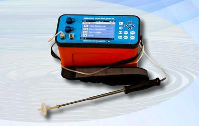
The comfortable shoulder strap allows for easy field work without fatigue. The probe makes it easy to measure the areal distribution of mercury concentrations.
